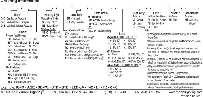
MR16 Remote Sealed Ingrade MODEL IG4 12V 42W Max., MR16 Halogen
